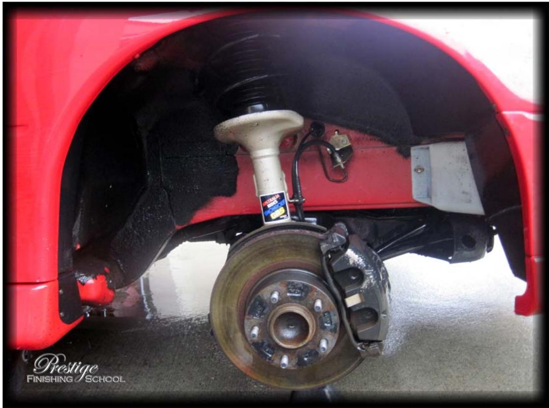
Although an underseal has been applied to the bulk of the wheel arches, a small plastic liner is still fitted – this is dressed with Meguiars All Season Dressing, leaving a very smart finish.
